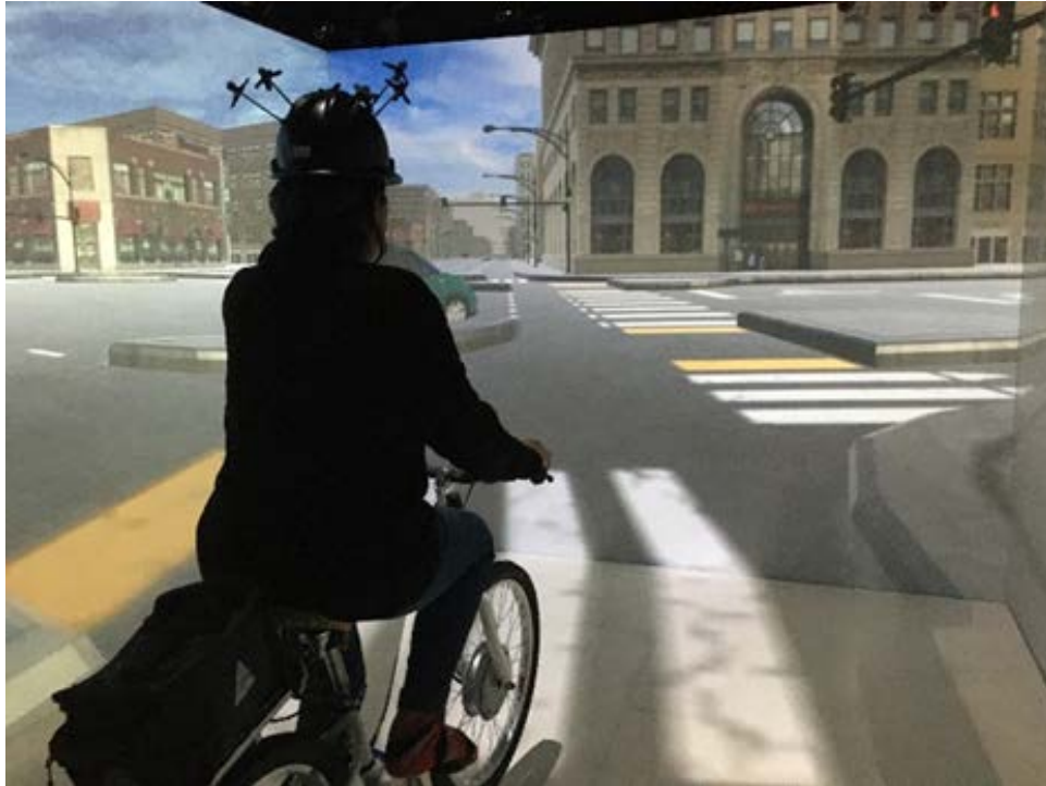
Figure 1.1 - A rider approaching a protected intersection in the bicycling simulator.
